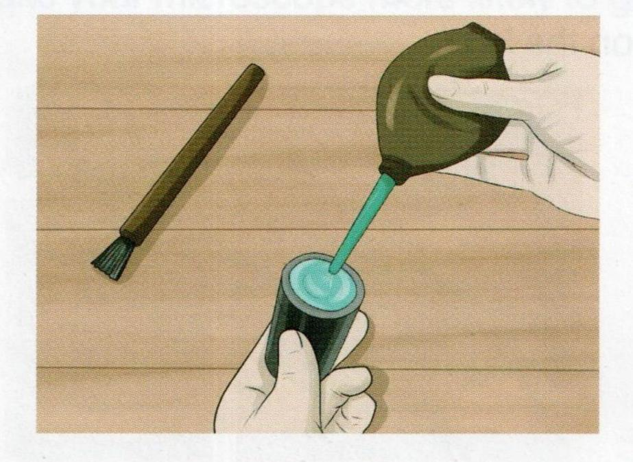
2. Spray oil-free compressed gas on the lenses to avoid damaging them. Using compressed air or gas is the best way to easily remove dust from your optical lenses if you don't have a dust brush or vacuum. However, do not use a compressed air product that contains solvents, as these will cause more harm than good to your lenses.
