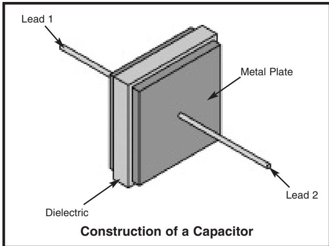
The dielectric is the material that holds the electric charge (pressure), just like the rubber diaphragm holds the water pressure. Some dielectrics may be thought of as stiff rubber, and some as soft rubber. The capacitance and working voltage of the capacitor is controlled by varying the number and size of metal-dielectric layers, the thickness of the dielectric layers, and the type of dielectric material used.
