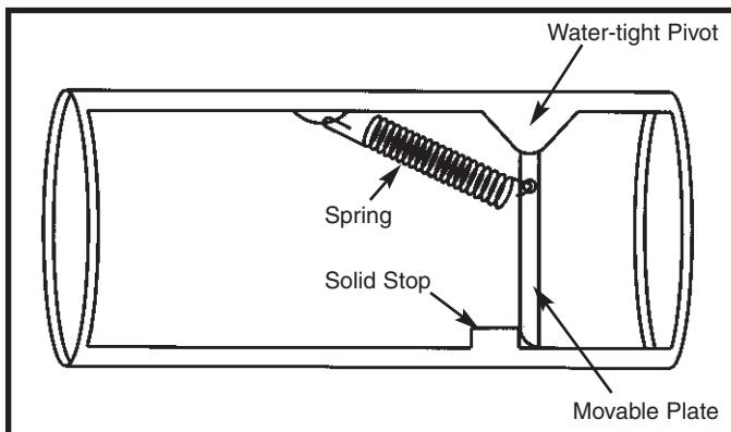
The check valve only allows water to flow in one direction, to the right in this drawing. There is a small spring and if the water pressure exceeds a certain level then the spring will be stretched and the valve opened. If the pressure is to flow to the left then the plate will be pressed against the solid stop and no water will flow.
