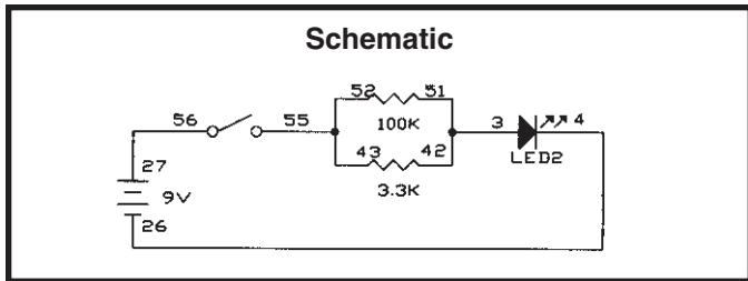
For two  $10\text{K}\Omega$  resistors in parallel, the result would be  $5\text{K}\Omega$ . The  $3.3\text{K}\Omega$  and  $100\text{K}\Omega$  in parallel in our circuit now give the same LED brightness as a single  $3.2\text{K}\Omega$  resistor.
