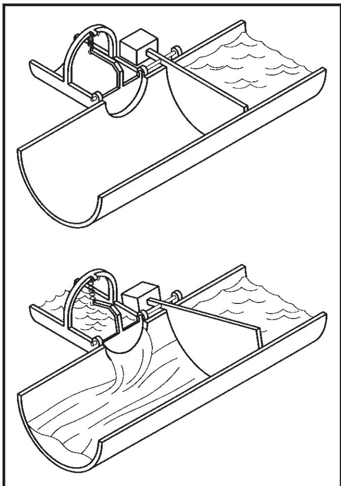
What would happen if the base and collector were connected together? Once there is enough pressure to overcome the spring in check valve DE (0.7V) there would be only slight resistance and no current gain. This situation should sound familiar since this is exactly how a diode operates. When the base and collector of a transistor are connected together the transistor becomes a diode.
