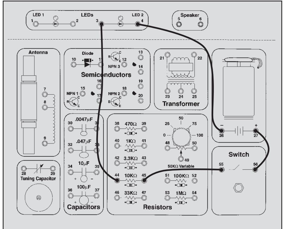
Press the switch (next to springs 55 and 56) and the **LED** (**light emitting diode**) lights up, and turns off when you release the switch. The LED converts electrical energy into light, like the light bulbs in your home. You can also think of an LED as being like a simple water meter, since as the electric current increases in a wire the LED becomes brighter. It is shown here, with its symbol.
