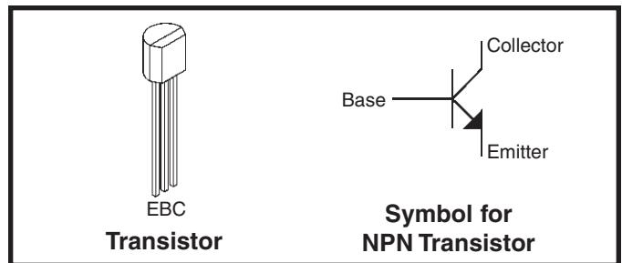
Note the small arrow in the emitter, this indicates which direction the current will flow through the device.
