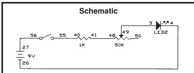
Now remove the wire from spring 49 and connect it to spring 48. What do you think will happen? Close the switch and turn the dial. The LED is dim and turning the resistor dial won't make it any brighter. As discussed above, the resistance between 48 and 50 is always  $50\text{K}\Omega$  and the part acts just like one of the other resistors in your Electronic Playground.
