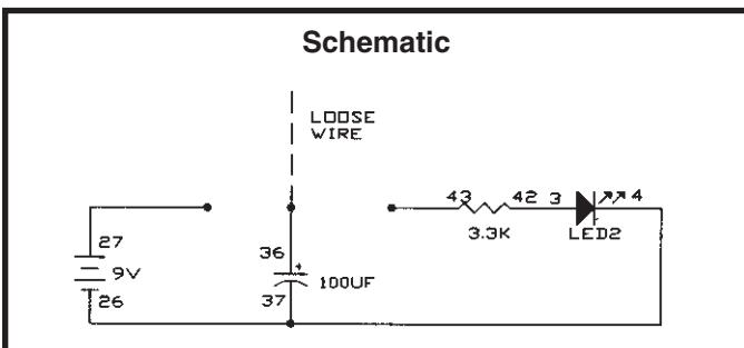
in place of the  $3.3K\Omega$ ; lower values will make the LED brighter but it will dim faster while with higher resistor values the LED won't be as bright but it will stay on longer. You can also put a resistor in series with the battery when you charge the capacitor, then it will take time to fully charge the capacitor. What do you think would happen if you used a smaller capacitor value?
