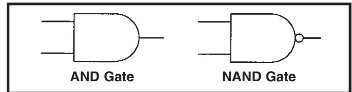
Combinations of AND and OR gates are used to add and multiply numbers together in computers. The additional use of NOT, NOR, and NAND gates allows a computer to represent any input/output pattern you can think of. By combining these gates with the memory and timing control that flip-flops provide, today's computers are created.
