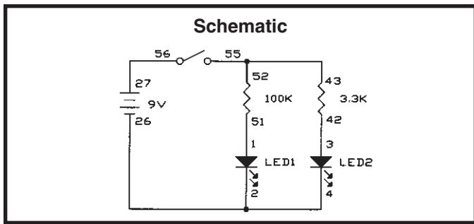
Replace the  $100\text{K}\Omega$  resistor with several values as before (such as  $1\text{K}\Omega$ ,  $10\text{K}\Omega$ , and others if you wish), pressing the switch and observing the LEDs each time. The brightness of LED2 will not change, but the brightness of LED1 will depend on the resistor value you placed in series with it.
