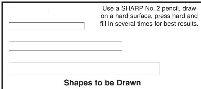
Actually, your pencils aren't made out of lead anymore (although we still call them "lead pencils"). The "lead" in your pencils is really a form of carbon, the same material that resistors are made of. So the drawings you just made should act just like the resistors in your Electronic Playground.
