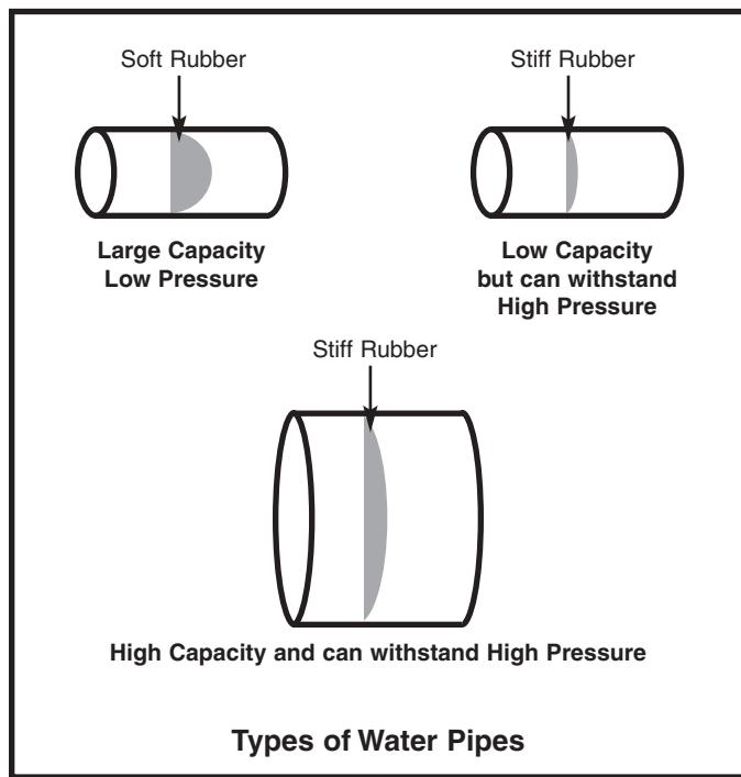
Similarly, capacitors are described by their capacity for holding electric charge, called their **Capacitance**, and their ability to withstand electric pressure (voltage) without damage. Although there are many different types of capacitors made using many different materials, their basic construction is the same. The wires (leads) connect to two or more metal plates that are separated by high resistance materials called **dielectrics**.
