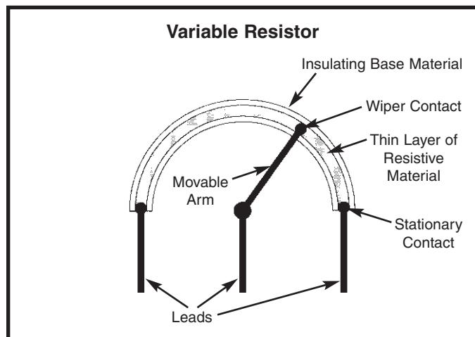
There is a scale printed next to the dial on the variable resistor which shows the percentage of the total resistance that is between springs 49 and 50. The remaining resistance will be between springs 48 and 49. The resistance between springs 48 and 50 will always be  $50\text{K}\Omega$ , the total resistance.
